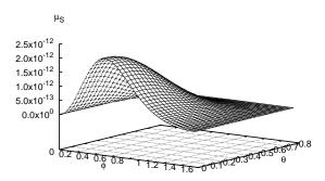
FIG. 12: Dependence of power conversion efficiency coefficient  $\mu_S$  on angles. "To the vehicle". Pumping frequency 12GHz.
