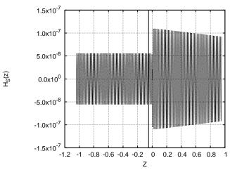
FIG. 9: Magnetic field profile of the Stokes wave. Pumping frequency 18GHz.
