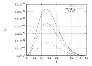
FIG. 15: Dependence the of power conversion efficiency coefficient  $\mu_S$  on several pumping angles, in the "to the vehicle" case. Pumping frequency 18GHz.
