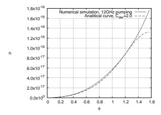
FIG. 16: Dependence of the power conversion efficiency coefficient  $\mu$  on optimal angle. "From the vehicle". Pumping frequency 12GHz.
