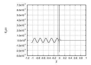
FIG. 7: Incoming signal electric field (z-component) profile.
