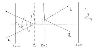
FIG. 1:  $\omega_L(z_r) = \omega \cos \phi$ ,  $\omega_L(0) = \omega$ . If the thickness of the plasma sheath is equal to L + R = 1m, the signal frequency f = 2GHz and the plasma frequency  $f_L \simeq 9GHz$  then  $L \simeq 5cm$  and  $R \simeq 95cm$ .
