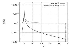
FIG. 5: The full right hand side (absolute value) of the Ginzburg equation in the "from the vehicle" case (solid line) together with the expression used in the approximation (dashed line). Logarithmic scale. Before the vicinity of point z=0 almost no forcing is present. Almost all contributions in the vicinity of the resonant point comes from the term used in the approximation. In the propagation region (z<0), the approximation slightly underestimates the right hand side.
