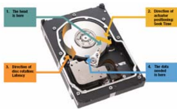
Figure 1: an example of a Hard Drive's standard internal components.
