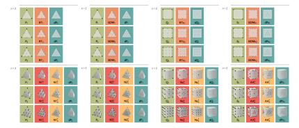
Classification of many common conforming finite element types.
