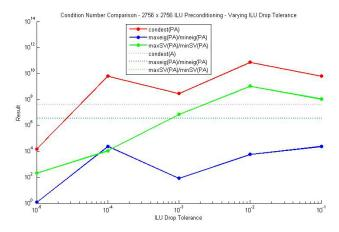
As was shown in the preliminary report, ILU preconditioning can be used to arbitrarily lower the number of required GMRES iterations, so we sought to find an optimal drop tolerance which weighs the memory needs of ILU versus GMRES, and minimizes the amount of computation time. In order to do this,
