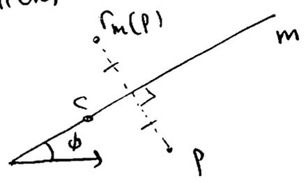
$$\Gamma_m(z) = z_{2\phi}(\overline{z-c}) + c$$
