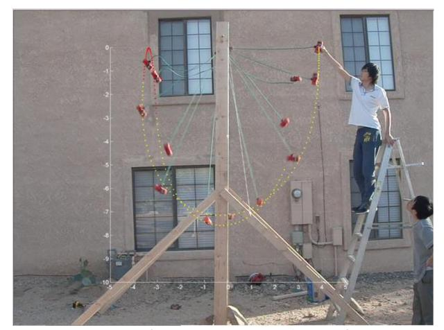
The mass is released from rest positioned horizontally at the characteristic length of the bungee.  $x_0 = 3.875$  feet
