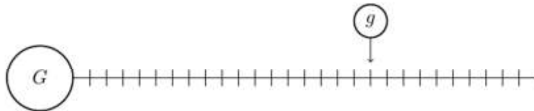
Figure 1: A diagram of a distribution line with a renewable source injecting power at some point in the line
