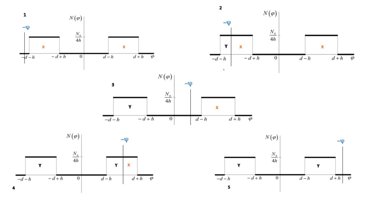
$$\frac{d\psi}{dt} = A\alpha \left[ C \left( 2 \int_{-\psi(t)}^{\infty} N(\varphi) d\varphi - N_0 \right) + b_1 - b_2 \right] - a\psi$$
