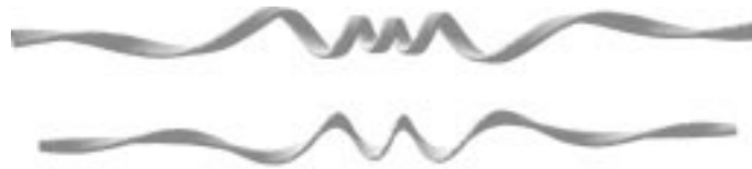
Fig. 5. The two localized exact solutions. The first one is a Kovalevskaya rod, that is a binormal homoclinic solution (top), the second one is a normal homoclinic solution (bottom).
