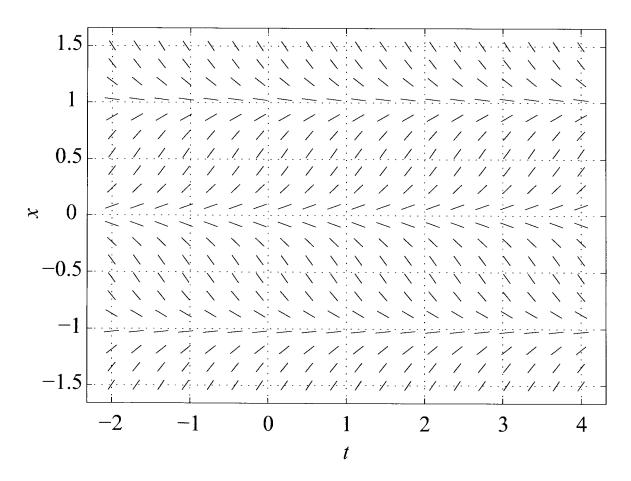
This slope field has equilibria at x=-1, x=0, and x=1. Both x=-1 and x=1 are stable, and x=0 is unstable.
