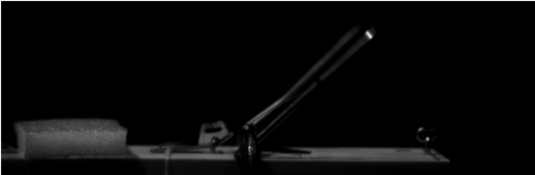
Fig. 10. This is the conventional rat trap in the process of being triggered. The tip of the bar is traveling at about 15 meters per second, about 25 milliseconds after it was triggered. By the time it reaches the shock absorber (left) at the end the tip will be moving about 30 meters per second.
