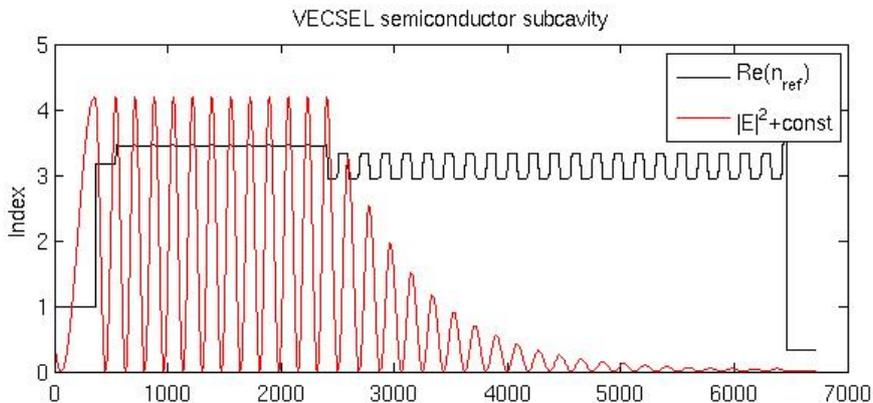
Figure 1: Structure of the active mirror in a VECSEL, showing the DBR (the periodic structure on the right) and the quantum well stack (in the left half of the image). Notice that the incoming light wave is intensified slightly as it moves through the quantum well stack, and decreases exponentially as it goes deeper into the DBR.
