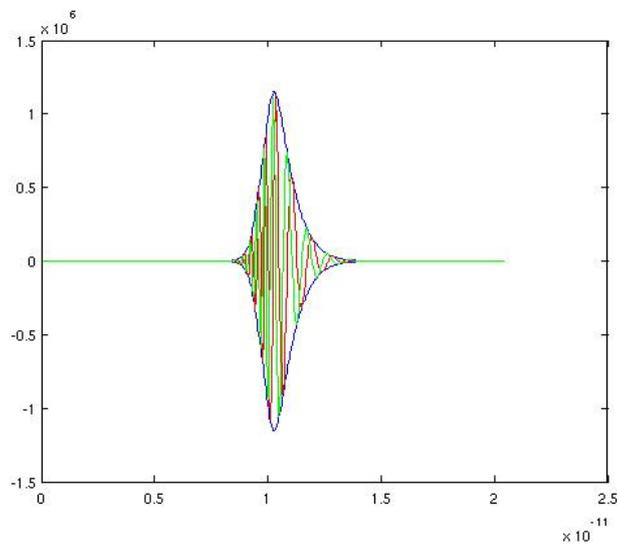
(b) Pulse generated by reference mirrors, 1.38 ps fs
