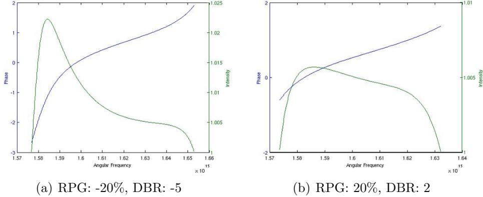
Figure 5: Examples of the effects of chirping both the DBR and the RPG structure
