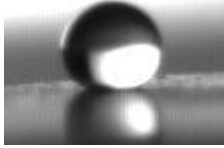
Figure 1: A drop with diameter 2.6mm rests on a super-hydrophobic surface. Note the high contact angle, which was measured to be 147 degrees.
