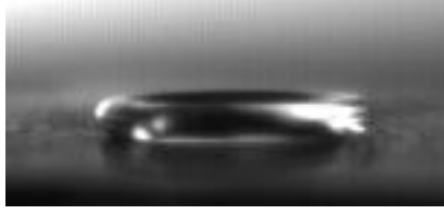
Figure 4: The shape of the drop at maximum spread resembles a gravity puddle because of its deceleration. The original diameter was 2.77mm and impact velocity .947m/s, giving We=17.2 . The maximum deformation (seen here) is 5.123mm
