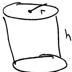
$$\text{Cost} = \text{Cost of Top} + \text{Cost of Bottom} + \text{Cost of Shell}$$
